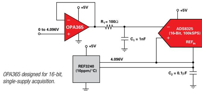
OPA365 designed for 16-bit, single-supply acquisition.
