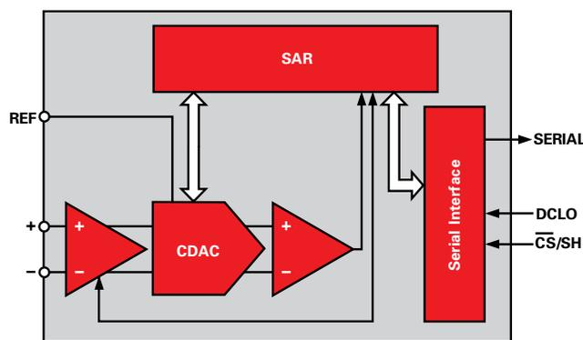
*In a SAR ADC, the bits are decided by a single high-speed, high-accuracy comparator bit by bit, from the MSB down to the LSB. This is done by comparing the analog input with a DAC whose output is updated by previously decided bits and successively approximates the analog input.*
