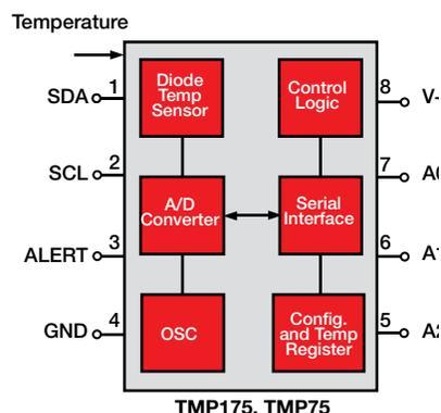
Typical block diagram of the TMP family of digital temperature sensors.
