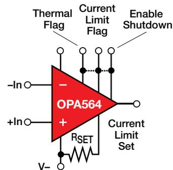
OPA564 PowerPAD™-down pinout.
