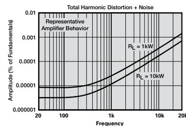
All these measures are made by applying a pure sine wave (or combination of sine waves) and measuring the spectral content in the amplifier's output that are not present in its input signal.
