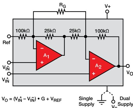
*Two-op-amp topology provides wider common-mode range in low-voltage, single-supply applications.*
