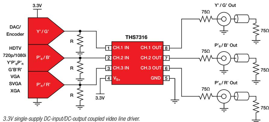
3.3V single-supply DC-input/DC-output coupled video line driver.
