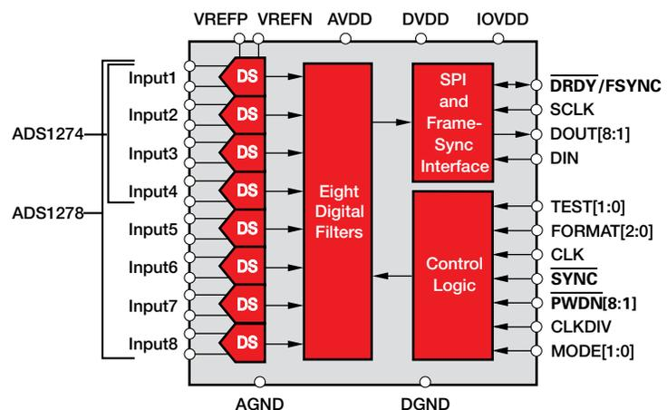
ADS1274 and ADS1278 functional block diagram.
