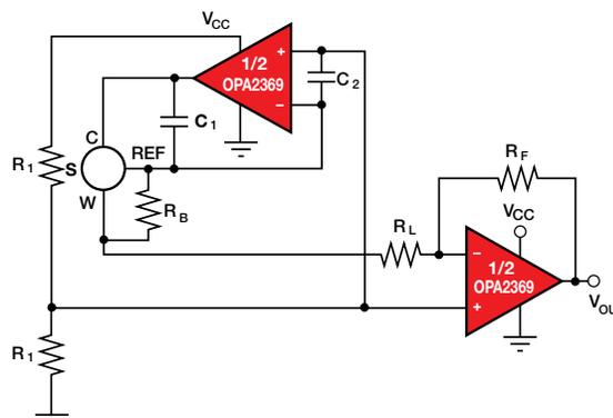
OPA369 as low-power gas-detection circuit.
