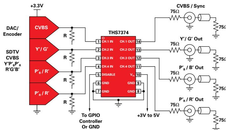
Figure 1. 3.3V Single-Supply DC-Input/DC Output Coupled Video Line Driver
