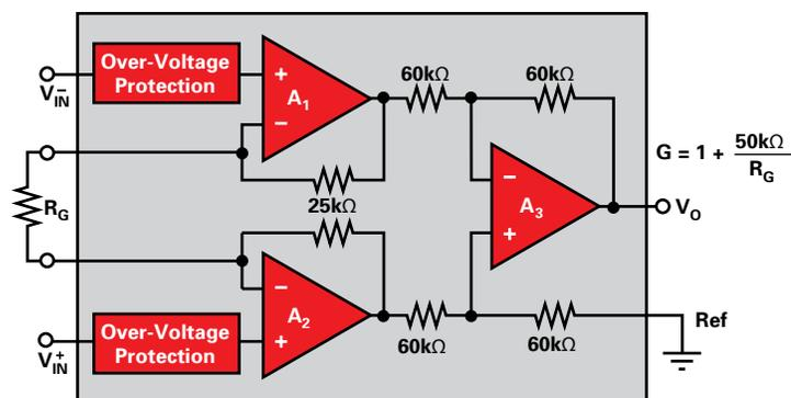
*The three-op-amp topology is the benchmark for instrumentation amplifier performance.*
