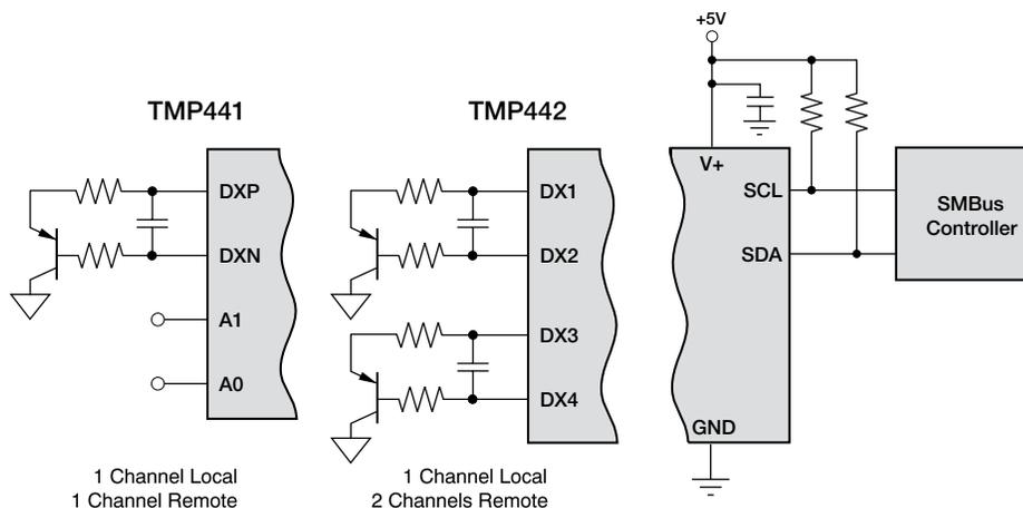
TMP441, TMP442 functional block diagrams. Estimated release date 4Q 08.
