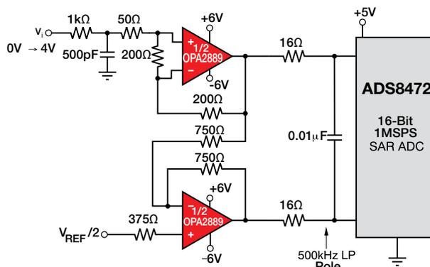
Low-power, DC-coupled, single-to-differential driver for ≤100kHz inputs.
