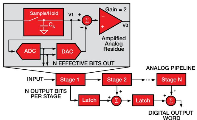
Pipeline ADCs consist of consecutive stages, each containing a S/H, a low-resolution ADC and DAC, and a summing circuit that includes an interstage amplifier to provide gain.
