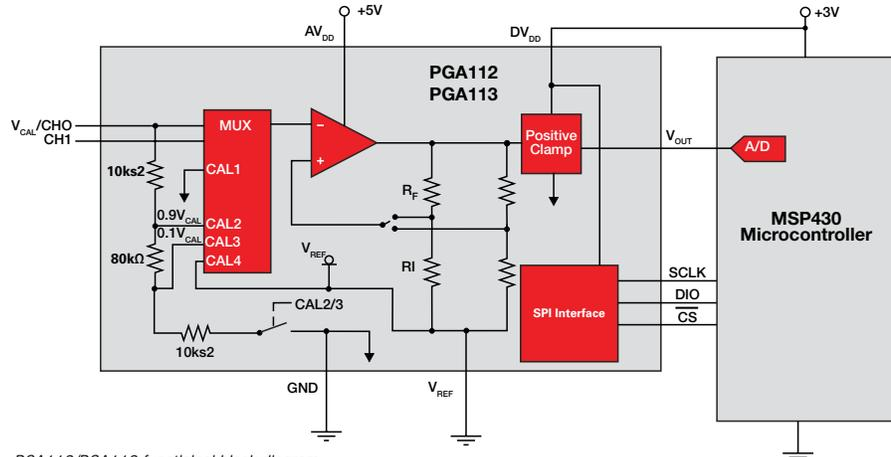
PGA112/PGA113 functional block diagram.
