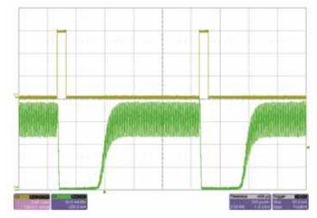
Output response to driving TP%. The input voltage was set to 12 V.
