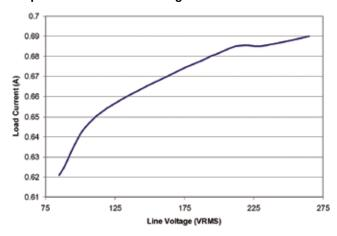
Load current as a function of line voltage. 10 Cree XLamp<sup>®</sup> 7090 XR-E, white, 700 mA LEDs connected in series was used for the load.
