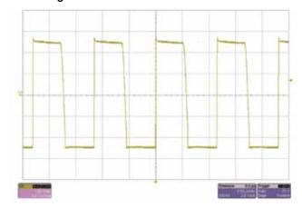
The image above shows the voltage on the anode of D1. The input was set to 250  $V_{\rm DC}$ .
