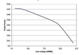
Power factor as a function of line voltage.10 Cree XLamp® 7090 XR-E, white, 700 mA LEDs connected in series was used for the load.
