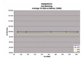
UCC28810EVM-003 I<sub>OUT</sub> matching vs. line voltage 4 x 15 Cree XRE LED's at 500 mA.
