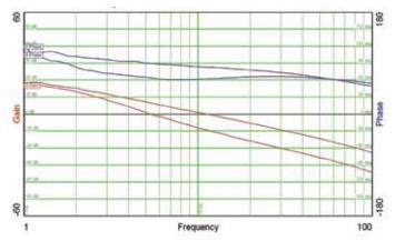
The frequency response of the feedback loop is shown in the plot above. The input was set to  $220\,V_{AC}$ . The lower gain plot was taken with a  $300\,V$  output. The upper gain plot was taken with a  $250\,V$  output.
