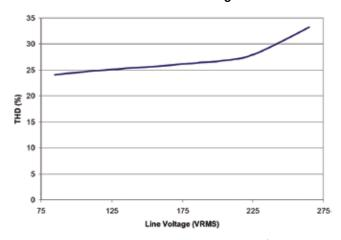
Total harmonic distortion as a function of line voltage. 10 Cree XLamp® 7090 XR-E, white, 700 mA LEDs connected in series was used for the load.
