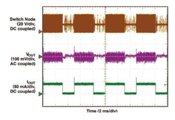
Mix Mode Dimming Current Linearity V<sub>IN</sub> = 10.8 V
