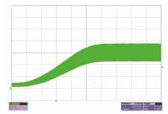
The input voltage was set at 12 V, with 0.15 (LED) + 1 (resistor) A load on the outputs.
