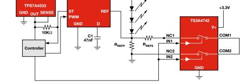
Figure 3. Analog-Switch Brightness Control
