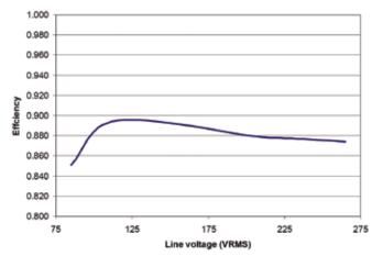
Efficiency as a function of line voltage. 10 Cree XLamp® 7090 XR-E, white, 700 mA LEDs connected in series was used for the load.
