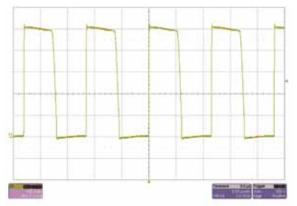
The image above shows the drain-to-source voltage on Q3. The input was set to 250.
