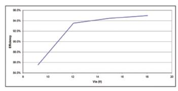
Total output current was 1.15 A, output voltage was 20 volts.
