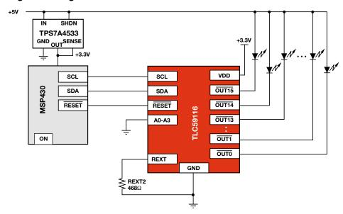
Figure 3. Analog Dimming/Blinking with a Load Switch
