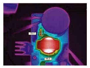
The image above shows a thermal image of the board. The ambient temperature was 26°C with no forced air flow. The input was 230  $V_{AC}$ .
