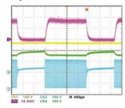
UCC28810EVM-002 transition mode buck PWM response. Ch1: Buck  $V_{\rm IN}$ , Ch2: Buck  $V_{\rm DS}$ , Ch3: LED current (0.5 A/Div), Ch4: LED voltage. Ch1 and Ch4 share GND reference.
