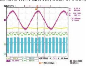
Ch1:  $V_{BUCK}$ +, Ch2: Buck  $V_{DS}$ , Ch3: AC line current 1A/Div, Ch4:  $V_{BUCK}$ - Ch1 and Ch 4 share GND reference.
