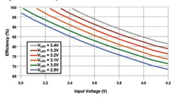
Figure 3 - LED Efficiency
